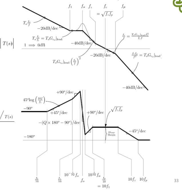
**Dominant Pole with Lead Compensation** Exact Bode plot for compensated loop gain ( $f_A = \frac{f_c}{33}$ ):
