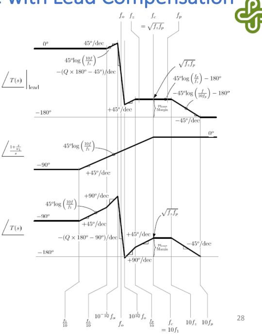
Asymptotic Bode plot for compensated loop gain |T(s)| $(f_A = \frac{f_c}{10})$ :
