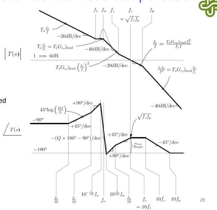
**Dominant Pole with Lead Compensation** Exact Bode plot for compensated loop gain ( $f_A = \frac{f_c}{10}$ ):
